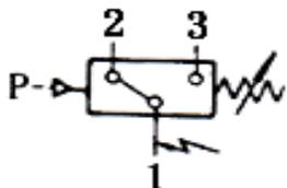
**Switching Function:****Micro-switch SPDT****Terminals 1-3: Contacts close on rising pressure****Terminals 1-2: Contacts open on rising pressure**
